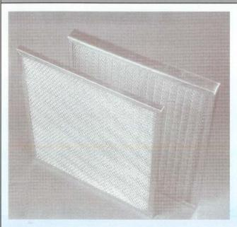
Tri-Dim's Mist Eliminator Filters are specifically designed to reduce airborne moisture including oil mist, water droplets, fog and other similar airborne contamination. Typical applications include outside air intakes, downstream of chilled evaporator coils and dehumidifiers. The Tri-Met ME is also extremely effective in areas where high or turbulent airflow conditions exist.
